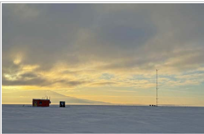
Elijah tall tower automatic weather station and hut near McMurdo. Photo by John Cassano.
