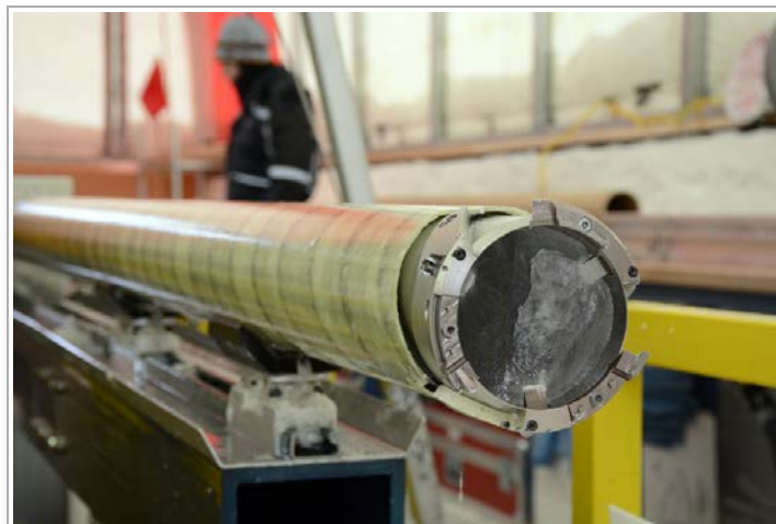
Drilling using the IDP ice-enabled Winkie drill for subglacial coring near Mt. Waesche during the 24/25 season. Photo by Nels Iverson.
