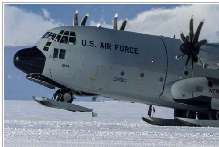
LC-130 aircraft taking off from Williams Field with the SCARGO sampling inlets above the cockpit. Photo by Mack Goodstein (NCAR).
